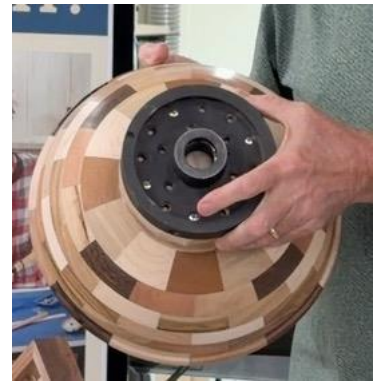
Figure 20 Mount blank to a face plate.
