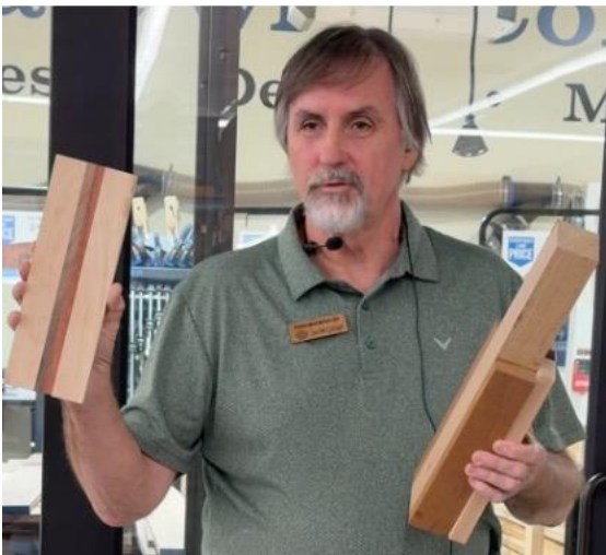
Figure 5 The core (left hand), with single pieces of wood glued to it.
