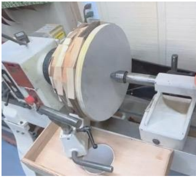
Figure 21 Tailstock end with plywood between bowl and tailstock center.
