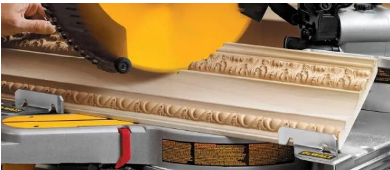
Figure 20 Nested on miter saw with crown stops.
