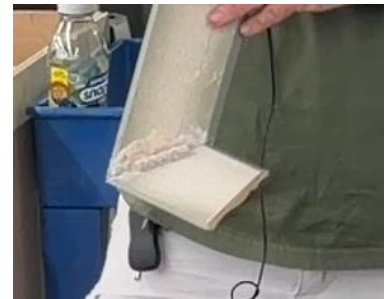
Figure 23 Dowel glued to mitered corner for support.
