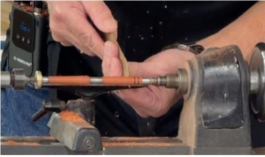
Figure 11 Grooving wood with another piece of wood
